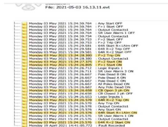
Gambar 5 Data Event Recorder Monitor Micom
