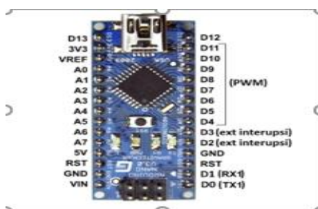
Gambar 2 Arduino Nano Pinout
