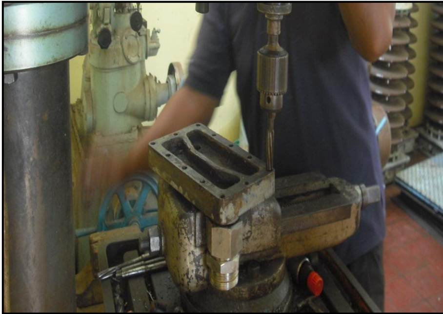
Gambar 4.6 Proses Mengebor Cover Cooler Turbine Guide Bearing
