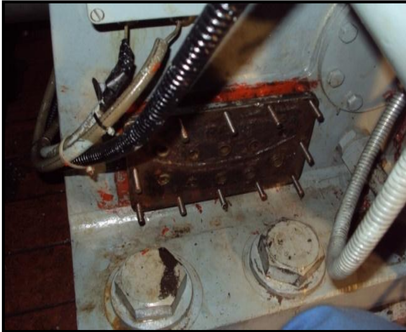
Gambar 4.8 Pemasangan Cover Oil Cooler Turbine Guide Bearing
